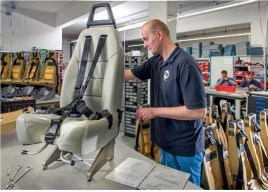
B/E Aerospace Fischer GmbH is a world leader in the sector of crash proof and extremely lightweight helicopter seats. They comply with the highest international standards and in the required stress tests even withstand a vertical application of force of 30 g (!). The company counts on Aalberts surface treatment's **hard anodizing (HART-COAT®)** for the coating of aluminum structural parts for the substructure.
