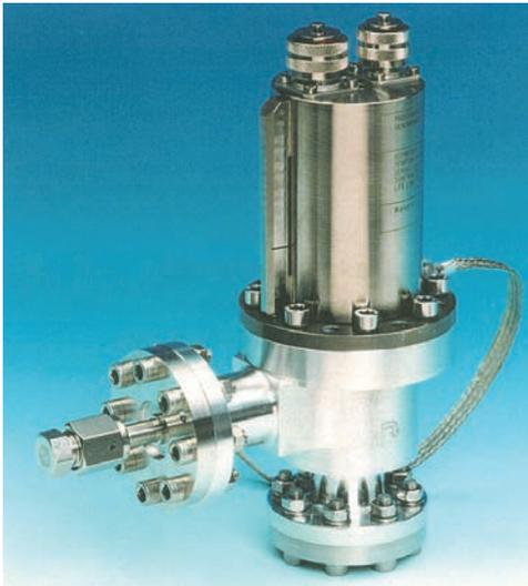
This check valve coated with **PTFE-DURNI-DISP** controls the supply of liquid helium. The coating offers very good adhesive wear resistance and outstanding dry running characteristics. It is heat-proof with excellent anti-friction and anti-adhesive properties and furthermore displays good corrosion resistance in combination with an intermediate layer. The dispersion layer combines valuable properties of **Electroless Nickel DURNI-COAT®** processing with the benefits of the fluoroplastic PTFE.
