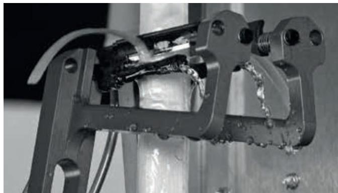
HART-COAT<sup>®</sup>-GLATT coated (25  $\mu\text{m}$ ) lever and knife carrier for asparagus peeling machines. The layer protects against corrosion and provides improved cleaning and wear properties.
