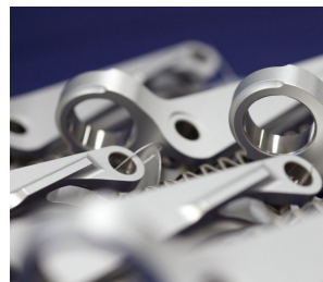
IVD coated components, with a masked internal diameter. The components have been treated with a trivalent chromate after application of IVD.
