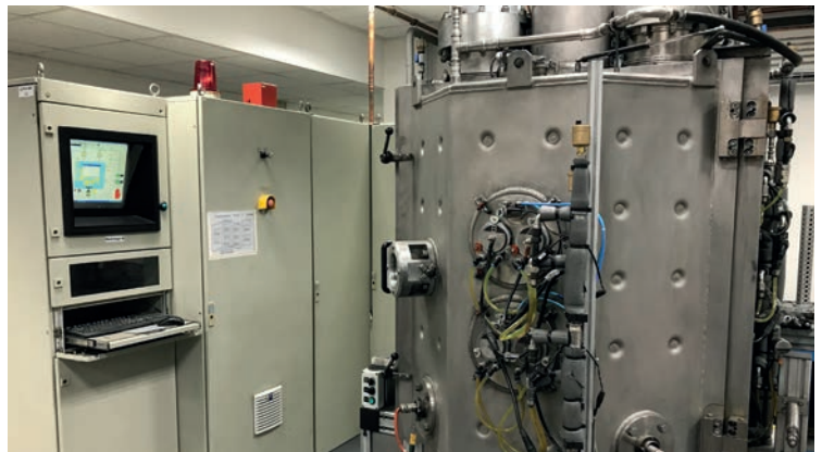
PVD system (working volume D 600 x 900 mm).
