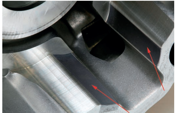
Aluminum workpiece with surfaces coated with the LASOX-COAT®-process.
