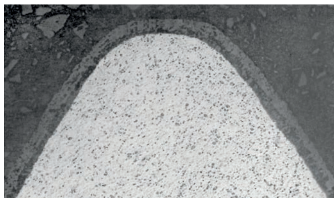
The photograph shows a metallographic microsection of a KEPLA-COAT® layer on a thread ridge.
