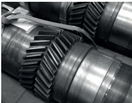
With molybdenum coated bearing seats of a drive shaft to prevent adhesive and abrasive wear.
