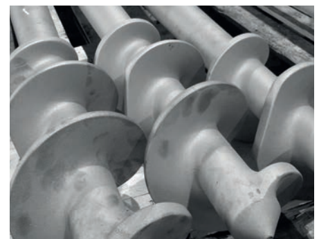
Wear protection of screw conveyors by flame spraying and smelting of a nickel hard alloy.
