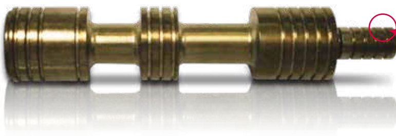
Valve spool, base material EN AW-6064 (AlMgSiBiPb), electroless nickel plated with the DURNI-COAT® process 571 (lead-free), heat-treated > 850 HV, before finish grinding.
