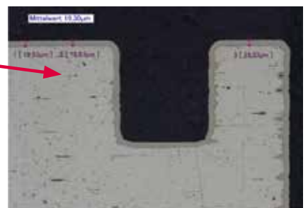
The valve spool was cut longitudinally for the micrograph (right). The area shown is circled red in the photograph. An even DURNI-COAT® layer envelops the component. Even complex component geometries can be coated with precise contours using DURNI-COAT®.
