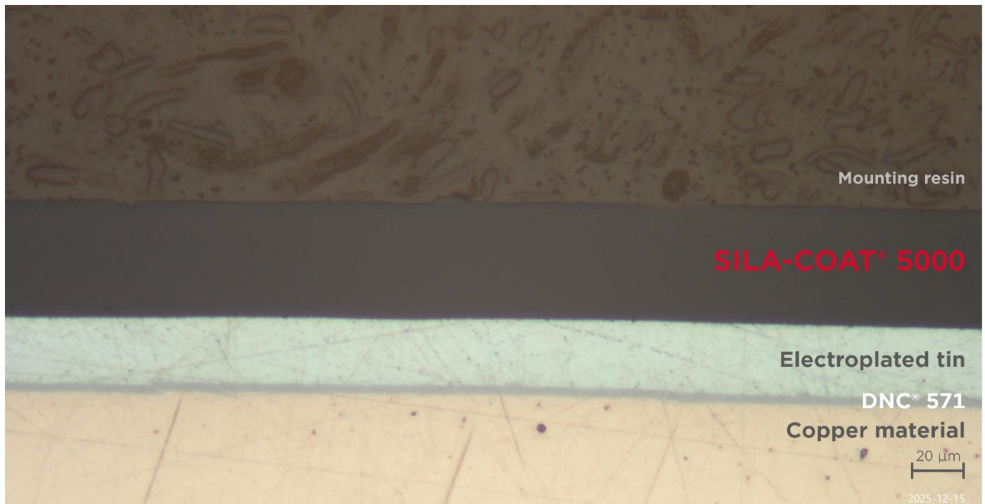
Figure 3: Copper material with a coating combination of DNC® 571 + electroplated tin + SILA-COAT® 5000
